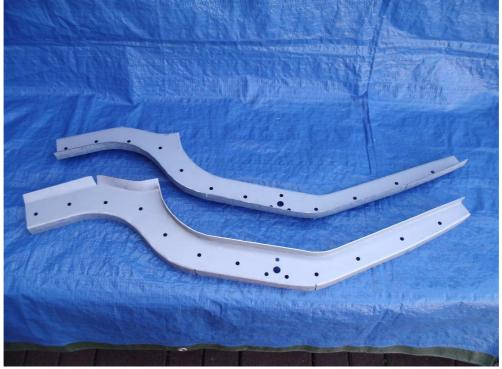
They are handmade from electrolytically zinc-plated steel-sheet.
