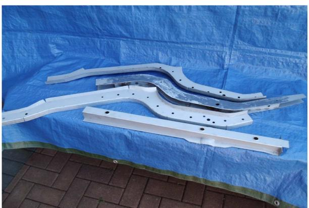
The straight part of the chassis leg is also handmade from 1,5mm electrolytically zinc-plated steel-sheet, price for one is 75€.
